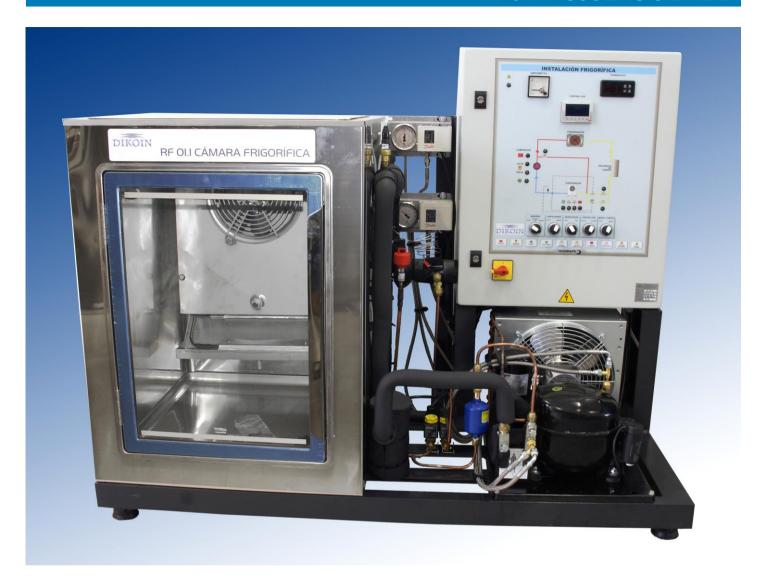
With this equipment, the industrial refrigeration phenomena is studied and visualized. It integrates all the essential components that a installation has in a bench top equipment. It is built with modular systems, and prepared for a freezing temperatures until -30°C.
